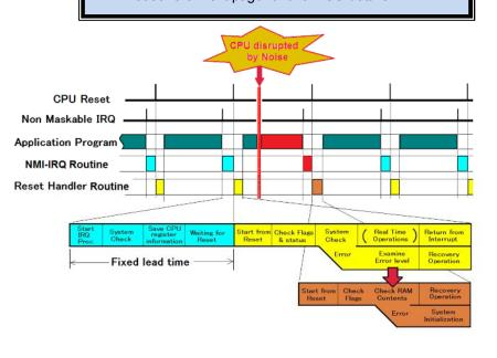
**FUJIMI technology** was invented and developed by LETech Co.,Ltd, Japan, and aimed at hot-start embedded MCU systems, enabling system operation to be continued after a malfunction without manual initialization. Error recovery can be handled in software with a high degree of flexibility. The technology is referred to as "High Resilience", and "FUJIMI" is a registered trademark.
